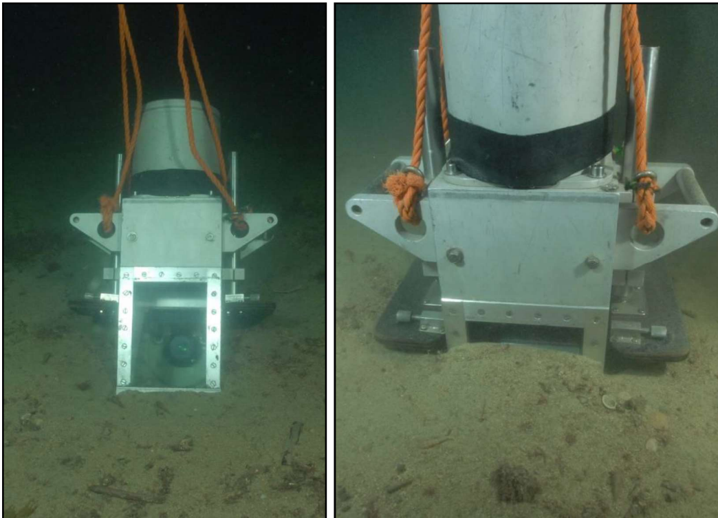
Figure 2.2: Diver operated Sediment Profile Imaging camera. The left-hand image gives a view of the camera at the sediment surface. The right-hand image shows the SPI camera when inserted into the sediment
